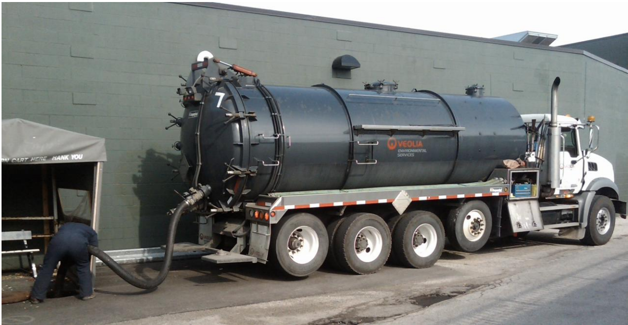
VEOLIA ENVIRONMENTAL SERVICES PUMPING SLURRY TANK
