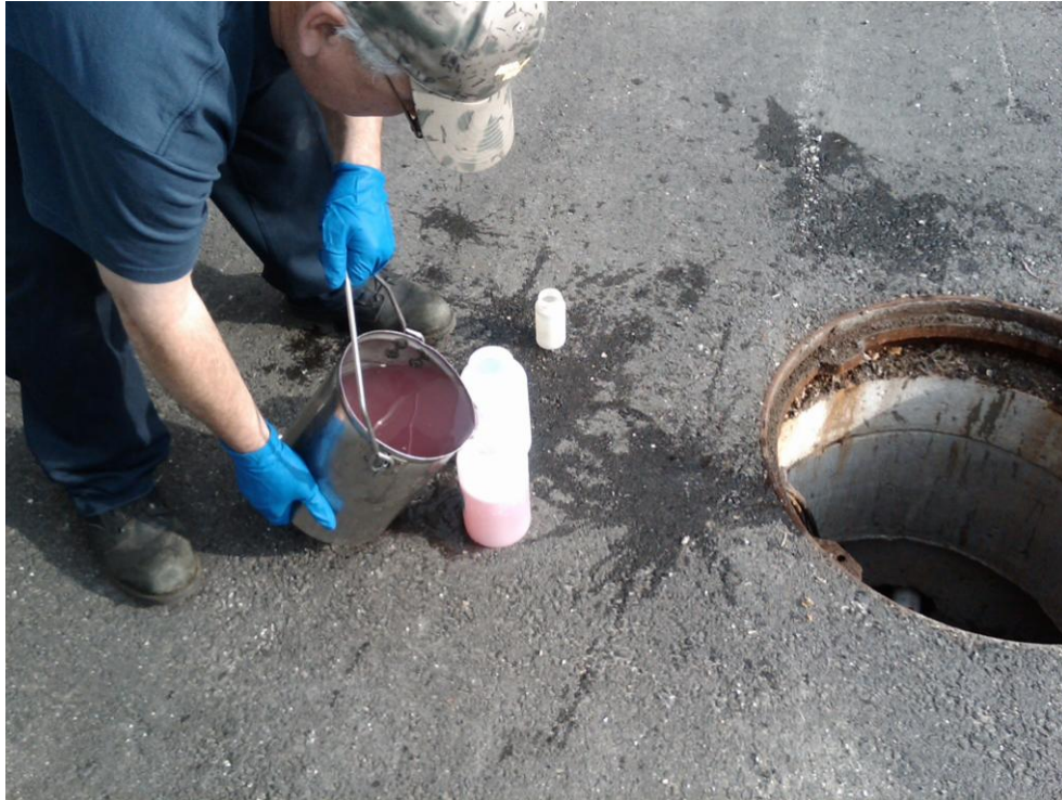
MMSD SAMPLING CREW COLLECTING SLURRY TANK EFFLUENT
